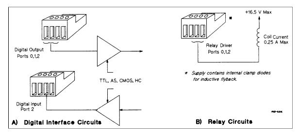
Figure D-5. Digital I/O Port Applications
